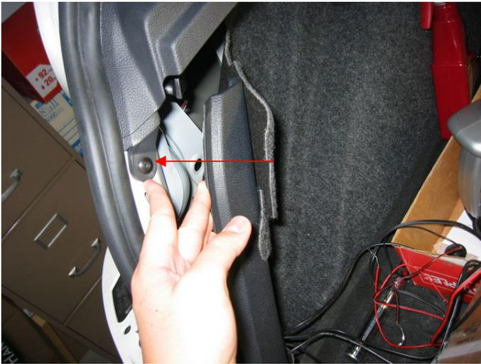
15. Remove the panel arrowed to below.
