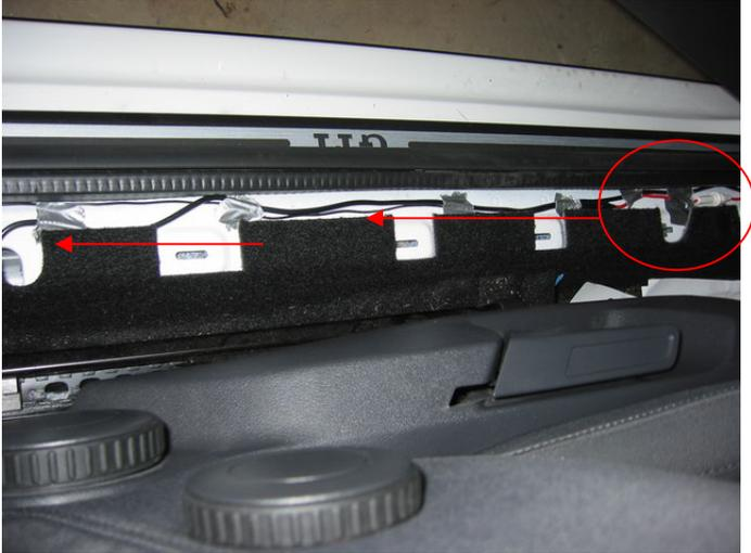
28. Run the snake down the side of the rear driver's side panel, under where the seat belt is. The snake should go in the direction as shown by the arrows, and will come out on the other side near the rear driver's side seat as shown in the pic to the right. If you don't get it right the first time, keep trying to feed the snake. It took me a few tries.
