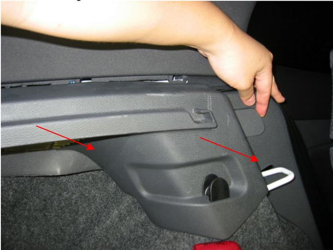
19. Here is the pic of the panel removed in Step #18. Arrowed to are the 3 plastic retaining posts that hold the panel piece on, in addition to the screws that were removed in Steps #14 & 17.
