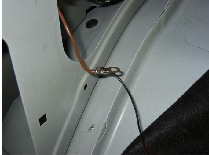
43. Connect the back-up light power wire from Step #8 and the ground wire from Step #41 into the power harness for the back-up sensor kit, using either the soldering iron, or some butt connectors. My harness was simply two wires, so fairly straight forward.
