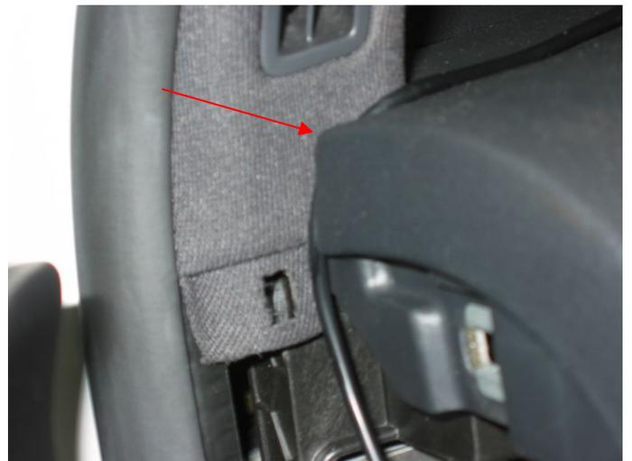
26. Push the hood release panel outward, and feed the wire through the panel, in the direction of the arrows.
