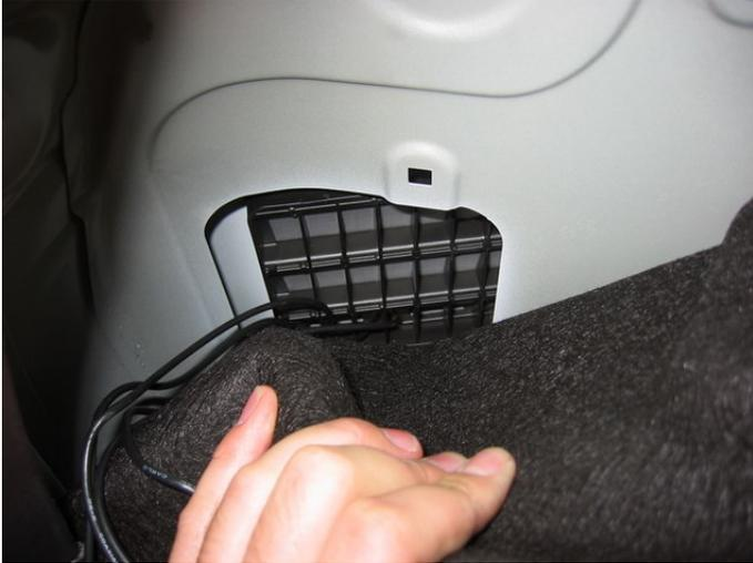
41. Re-attach the bumper following the rear bumper removal diy, making sure not to pinch any of the sensor wires.
