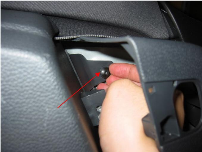
18. Pull the panel outward in the direction of the arrows to remove it. Also, see Step 18.
