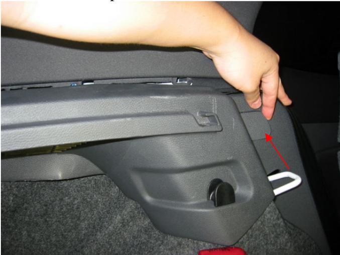
16. Use a T-20 driver to remove the screw behind the panel in Step #15. Pull the panel outward as arrowed below.
