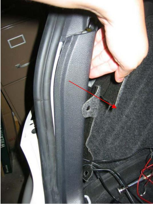
14. Use a T-20 driver to remove the screw that's behind the panel in Step #13.
